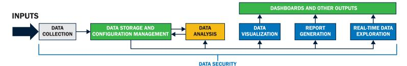
This illustration shows a high-level system block diagram ingesting data from multiple sources, structuring it into a common secure repository, then processing the data into actionable information.
